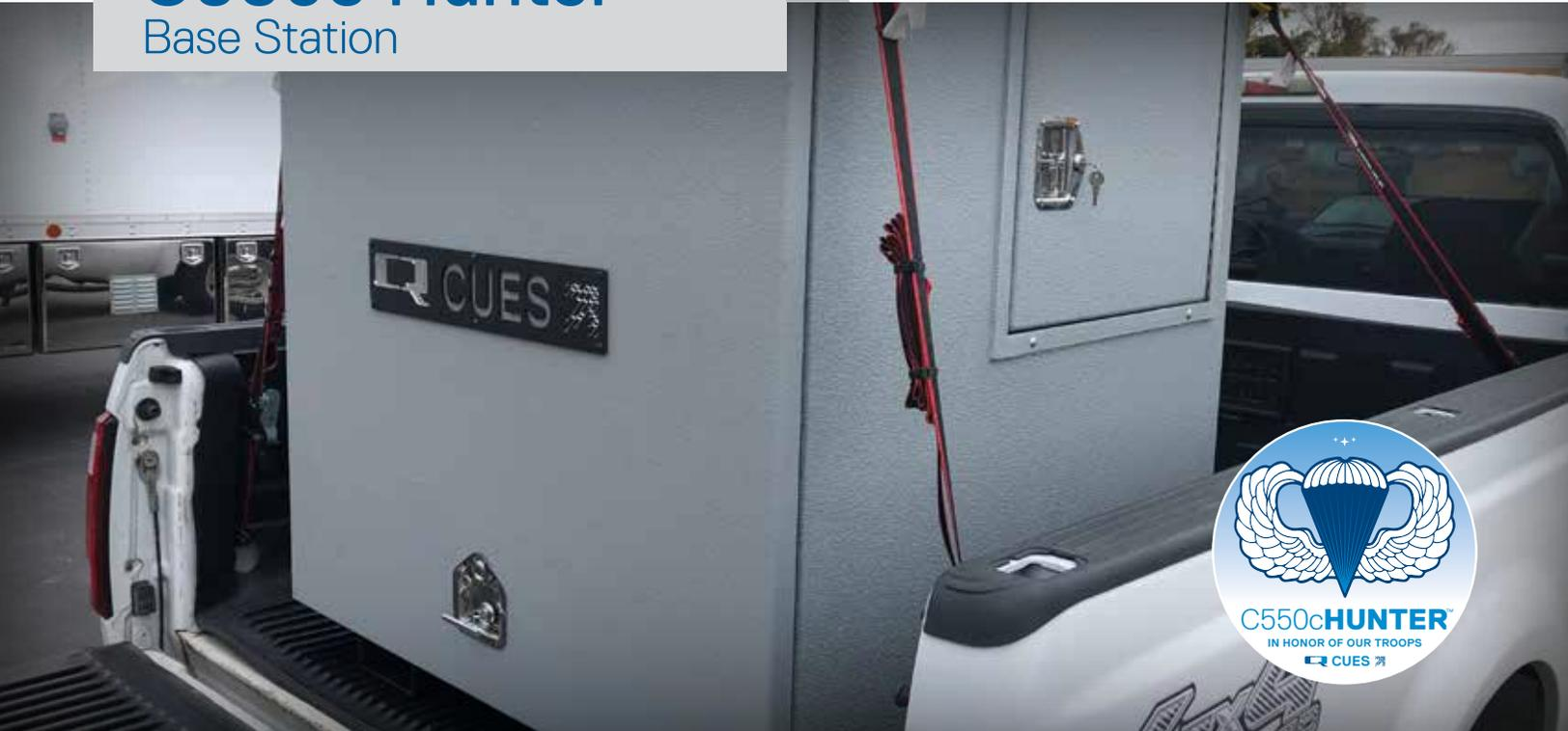
The CUES C550c Hunter is mounted in a compact and rugged weatherproof enclosure that can fit into an ATV, van, or pickup truck to access easements and hard-to-reach areas.
