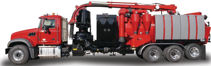
X-Vac is the top-of-the-line hydro excavator on the market. All X-Vac trucks offer a low profile debris tank for a lower center of gravity, variable control for pressure and flow that is separate from the blower RPM, and a dual cyclone separator with enlarged collection chambers.
